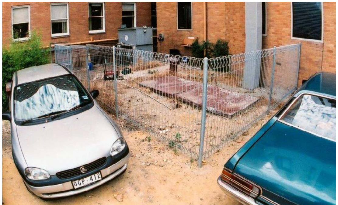
Environmental contamination: An unmaintained car park in the area adjacent to a cooling tower may increase the levels of solids in the water and must be addressed in the RMP
